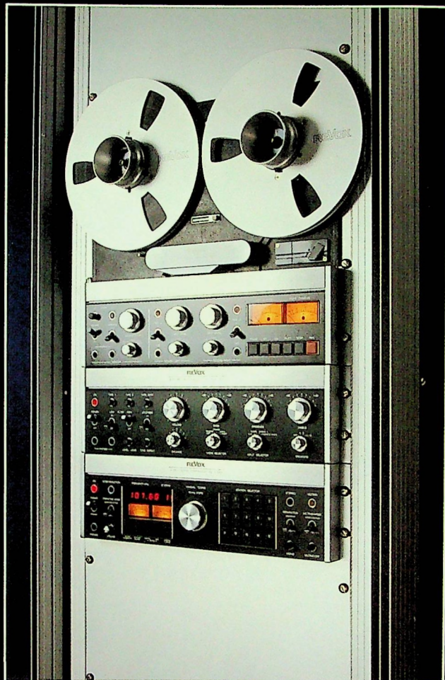
19" rack installation. Required for this is the CM model for panel mounting with metal case plus the 19" adapter kit, article no. 34099 (for B750 and B760 use article no. 34095).
