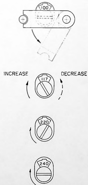
Fig. 5-17 Voltage Selector Setting
