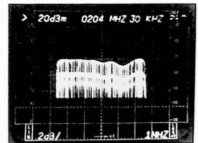
Figure 6-2. Swept heterodyne processor response.
