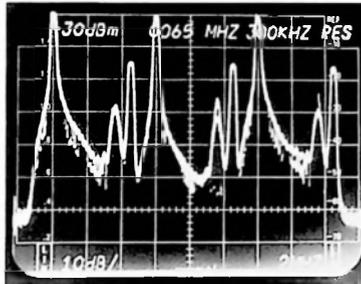
Figure 1-3. Amplitude measurements using the 7L14's digital storage.
