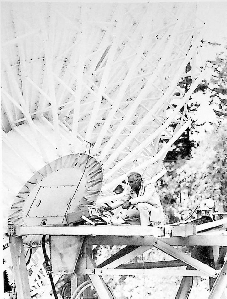
The Tek 492 Spectrum Analyzer measuring signals out of a 4 GHz antenna LNA. The 492 measures everything from baseband to satellite up/down link signals — at your headend, antenna site, or at a remote cable location.
