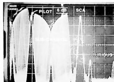
Fig. 5. Display of Composite Fm Stereo Signal on Low Frequency Spectrum Analyzer
