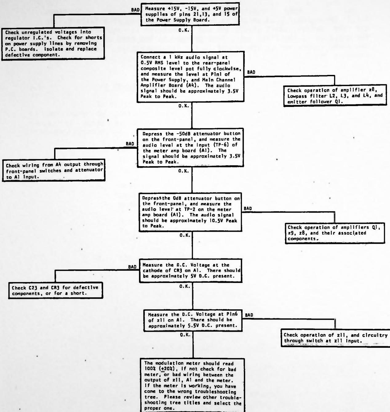
**5.7.2 Main Channel (L + R) does not work, but SCA Injection and SCA Modulation functions do work.**
