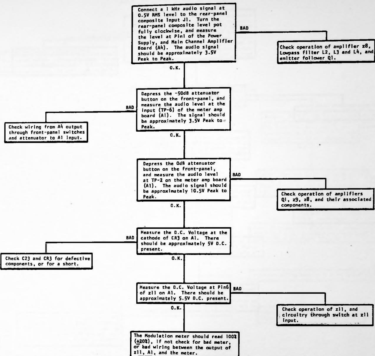
5.7.3 SCA injection does not work, but main channel (L + R) does work.
