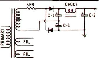
1SPR = Surge Protection Resistance required with a capacitive input filter.
