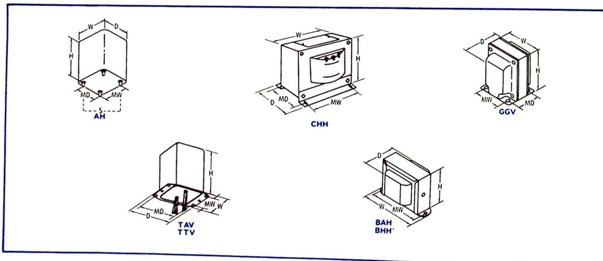
THORDARSON inductors provide total coverage of power supply and special application requirements. Smoothing, swinging, high current, toroidal, and alignaire variable inductors are listed in order of increasing current ratings. The rated inductance in henries of smoothing chokes can be varied slightly if the rated current is changed.
