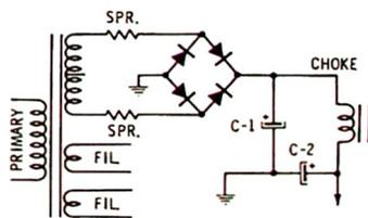
1SPR = Surge Protection Resistance required with a capacitive input filter.
