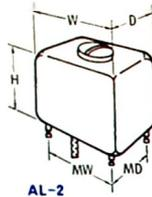
These Alignaire Inductors are ideally suited for hard to align or frequently changed circuits such as low frequency oscillators, attenuators, low frequency tuned amplifiers, filters and delay lines. The high frequency and temperature stability built into these units make them most applicable to mid-audio tuned frequency circuits.
