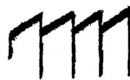
At junction of output winding of Vertical Output Transformer T1 and Vertical Yoke
