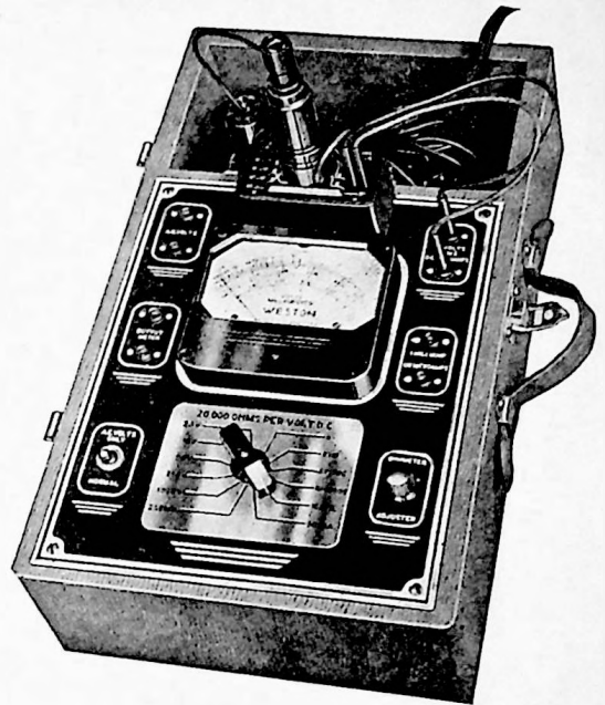
View Showing Model 666 Socket Selector Block Mounted on Model 772 Analyzer
