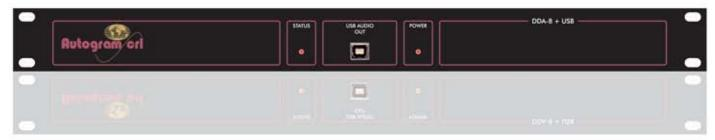
The DDA-8+USB is a high resolution, all digital, professional-grade 8 output digital audio distribution amplifier designed to isolate and distribute digital audio data formatted in accordance with AES/EBU specifications. The DDA-8 accepts a single digital audio input and transparently distributes the buffered signal on eight XLR outputs and on a USB port.
